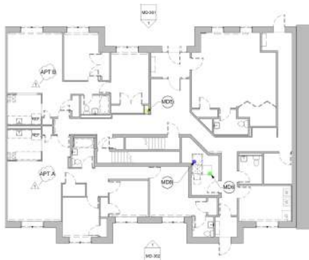
1 FIRST FLOOR DEMOLITION PLAN MECHANICAL SCALE: 1/8" = 1'-0"
